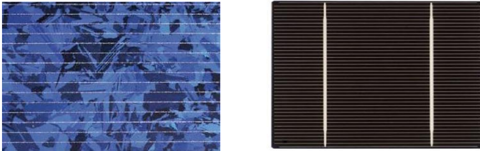
Figure 1-4 et 5: Cellule polycristalline et monocristalline [2]
